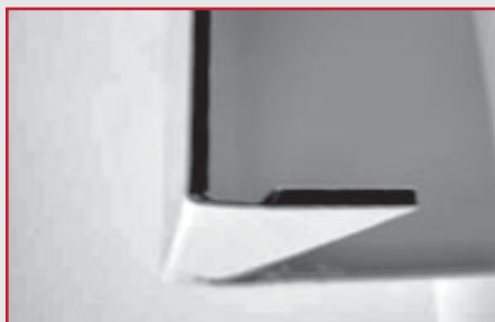
Distorted Flat Rout Folded 90°
