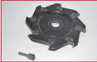
135° Router Bit & Saw Blade
